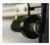
Front guide rollers are height adjustable to compensate for lane topography. Four heavy-duty ball bearing transport casters are aligned for enhanced stability on ramps.
