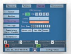
Multiple levels of security are available to control which machine functions can be accessed and adjusted by different users.
